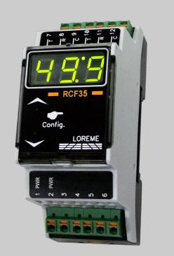
The RCF35 is a compact relay for monitoring the frequency variations on 50/60Hz and 400Hz networks. It can detects the over frequency and the under frequency event with the two independents thresholds setting. A LED display with 3 digits shows the network frequency measurement.
